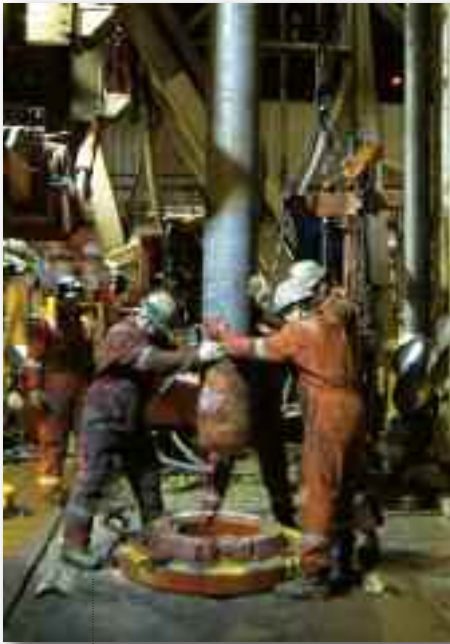
23 JULY 2010 ERNEST SPURRED LOWERING CASING THROUGH THE DRILL FLOOR
