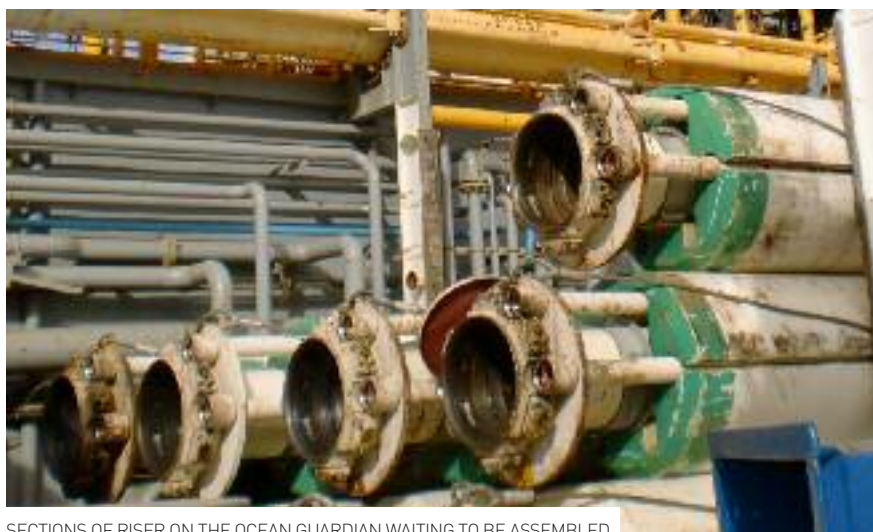
SECTIONS OF RISER ON THE OCEAN GUARDIAN WAITING TO BE ASSEMBLED
